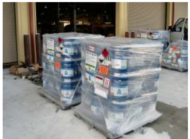
The Koester American ORS-C epoxy coating stored under the shed roof outside of door D in the back of the facility. Note that all pallets are properly marked and wrapped for safe shipping.
